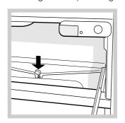
by the compressor causes it to evaporate. It is not, therefore, necessary to defrost the refrigerator manually. It is, however, necessary to clean the discharge hole regularly so that the water can flow out easily.
